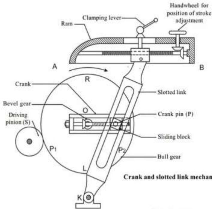
**Crank and slotted link mechanism**
