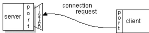
If everything goes well, the server accepts the connection. Upon acceptance, the server gets a new socket bound to the same local port and also has its remote endpoint set to the address and port of the client. It needs a new socket so that it can continue to
