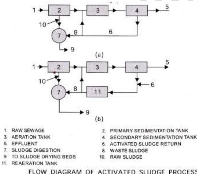
The primary effluent is mixed with a portion of returned sludge(activated sludge)and then allowed into the tank. This mixed liquor is then aerated or mechanically agitated in the presence of air. The aerobic bacteria kept in suspension oxidize the sludge. The oxidized sludge is withdrawn and send to secondary clarifier for sedimentation. The operation is a continuous process. The recycling of the returned sludge is shown in the fig.
