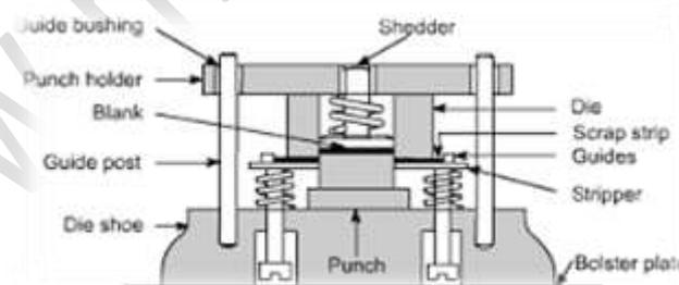
In inverted dies, the die is attached to punch holder and the punch is carried on the die shoe attached to the bolster. As the ram descends, the blank is cut off from the strip. On the upward stroke of the ram, the shedder pushes the blank out of the die opening and the stripper forces the scrap strip off the punch. Design of inverted dies is complicated and its cost is high. However, there is little possibility of thin blanks being bent, and the cutting edges need less regrinding.
