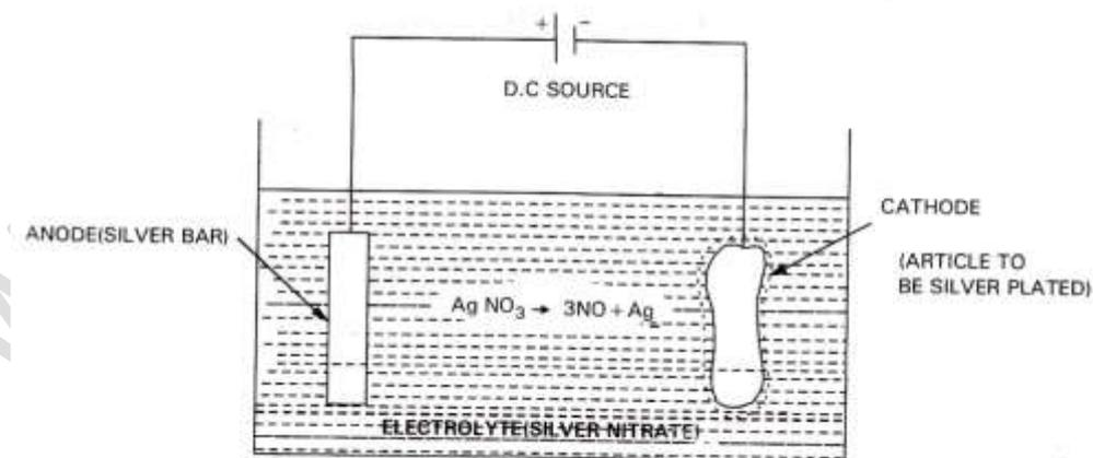
Fig. 11.1 PRINCIPLE OF ELECTRO - PLATING (SILVER-PLATING)
