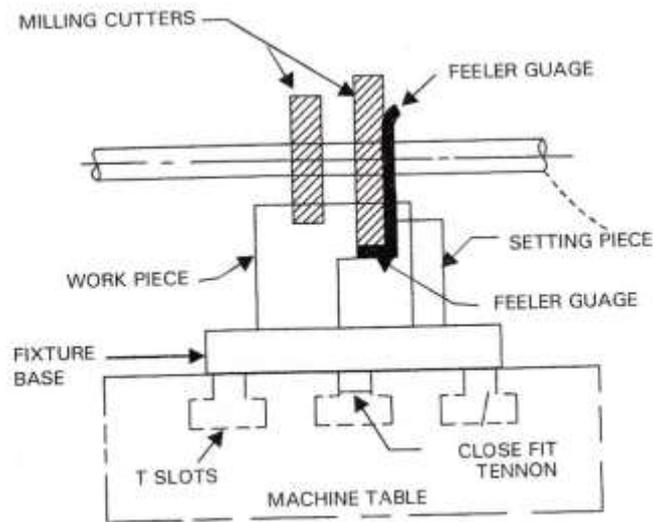
Fig. 8.10 (b) MILLING FIXTURE
