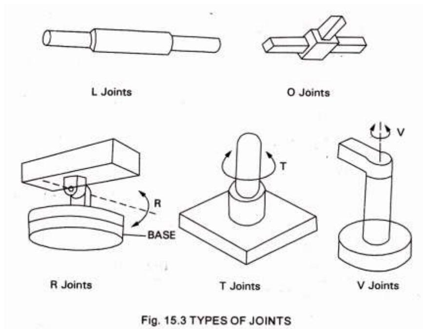
A joint permit the relative motion between two links or arms of robot. Various types of mechanical joints are,
