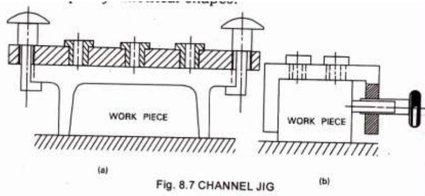
The body of channel jig is in the form of standard channel. The component is located in a channel and is clamped by screw. It is used for drilling simple symmetrical shapes.
