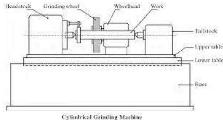
The plain cylindrical grinding machine shown in figure. It has the following parts,
