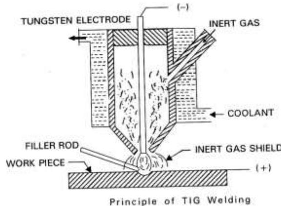
The shielding gases generally used are argon, helium or their mixtures. A separate filler rod is used to add filler metal. TIG welding is specially used for aluminums and its alloys.
