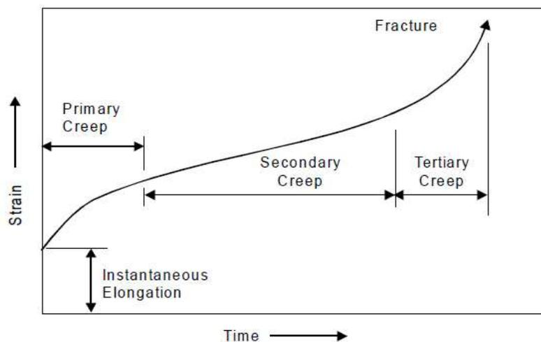
**Creep curve for high temperature and long time creep**
