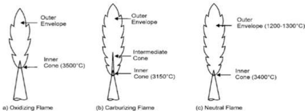
**Reducing flame:** It has an excess of acetylene over the oxygen. It has a longer inner cone, an intermediate feather and bluish outer flame. It is used for welding high carbon steel. The flame has carburizing effect on steel, causing hard, brittle and weak weld.
