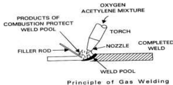
Oxy-acetylene flame is the most versatile and hottest of all the flames produced by the combination of oxygen and other fuel gases. Other gases such as Hydrogen, Propane, Butane, Natural gas etc., may be used for some welding and brazing applications.
