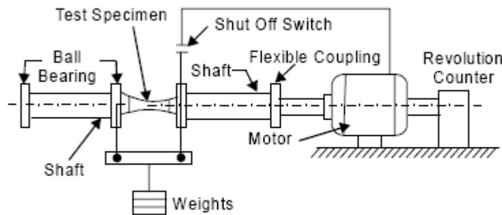
Fig. Schematic fatigue test setup
