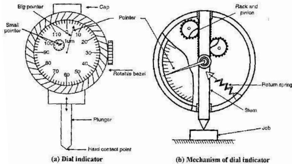
The movement mechanism of the instrument is housed in a metal case for its protection. The large dial scale is graduated into 100 divisions. The indicator is set to zero by the use of slip gauges representing the basic size of part.
