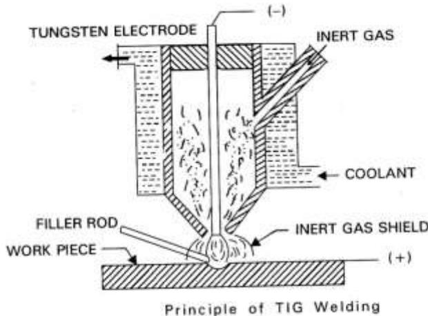
The shielding gas protects the tungsten electrode and the molten metal weld pool from the atmospheric contamination. The shielding gases generally used are argon, helium or their mixtures. TIG welding is specially used for aluminums and its alloys.
