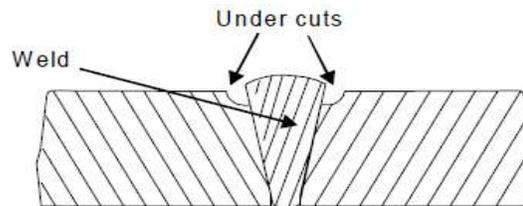
**(2) Undercut:** Groove formed along the edges of the welding bead, thereby reducing the thickness of base metal. It caused due to excessive current, excessive speed and wrong electrode position.
