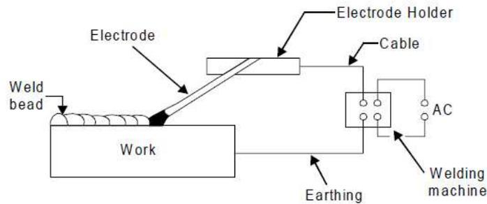
Fig. Principle of arc welding
