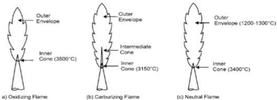
**Neutral flame:** It has equal quantities of oxygen and acetylene. It is most common flame used in welding processes. It has no tendency to react with material being welded.
