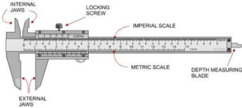
Fig. shows the Vernier caliper, which is commonly used to measure accurately
