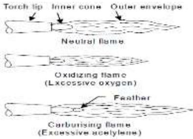
**Reducing flame:** It has an excess of acetylene over the oxygen. It has a longer inner cone, an intermediate feather and bluish outer flame. It is used for welding high carbon steel. The flame has carburizing effect on steel, causing hard, brittle and weak weld.
