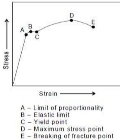
**Proportional limit:** It is the stress at which the stress-strain curve deviates from linearity. Upto this point, stress is proportional to strain.
