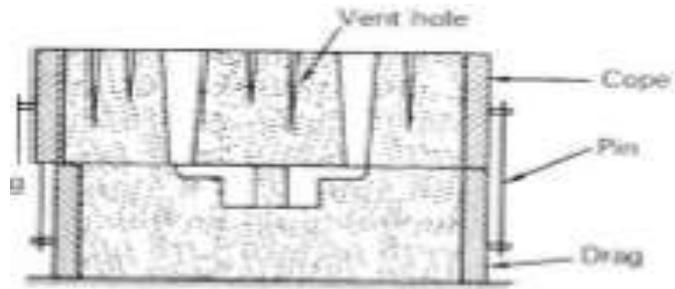
v) Cope placed on drag & vent holes are made. Mould is ready for pouring
