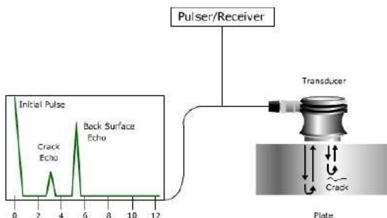
UT inspection system consists of several functional units, such as the pulser/receiver, transducer, and a display device. A pulser/receiver is an electronic device that can produce high voltage electrical pulses. Driven by the pulser, the transducer generates high frequency ultrasonic energy.
