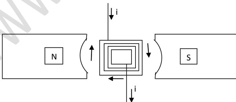
A rectangular coil of length 'l' and breadth 'b' is placed in a magnetic field B. the poles of the Magnet are made concave to produce radial magnetic field. Let a current 'i' experience any force as they are parallel to magnetic field. The length sides of the coil experience a force of Bil each acting in the opposite direction.
