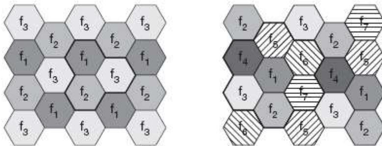
Cellular systems for mobile communications implement SDM. Each transmitter, typically called a **base station**, covers a certain area, a **cell**. Cell radii can vary from tens of meters in buildings, and hundreds of meters in cities, up to tens of kilometers in the countryside.
