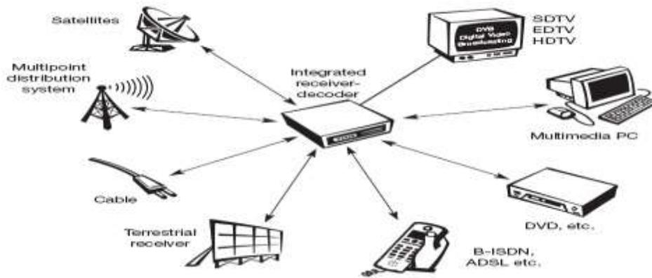
The center point is an integrated receiver-decoder (set-top box) connected to a high-resolution monitor. This set-top box can receive DVB signals via satellites, terrestrial local/regional senders (multi-point distribution systems, terrestrial receiver), cable, B-ISDN, ADSL, or other possible future technologies.
